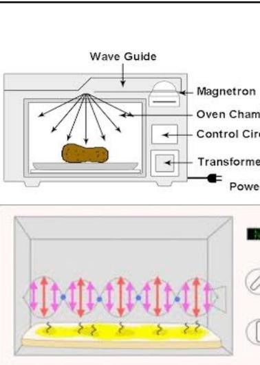
The diagram illustrates the internal components of a microwave oven: Wave Guide, Magnetron, Oven Chamber, Control Circuit, Transformer, and Power. It also shows a standing wave pattern of microwaves inside the oven chamber, with 'Anti-Nodes' labeled as 'maximum heating' and 'Nodes' labeled as 'no heating'.
